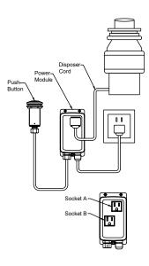
Plug the disposer cord in the power module.
