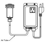
Attach air tubing between the push button and power module.
